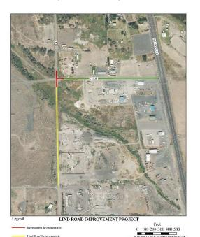
The City has identified a need to make improvements to Lind Road and Union Street in order to provide access to the Bonney industrial site. Currently, Lind Road is a gravel road while Union Street is paved but it does not meet industrial standards such as required road base depth, compaction depth, asphalt depth, compaction, and strength. Neither holds up to weather and traffic.
