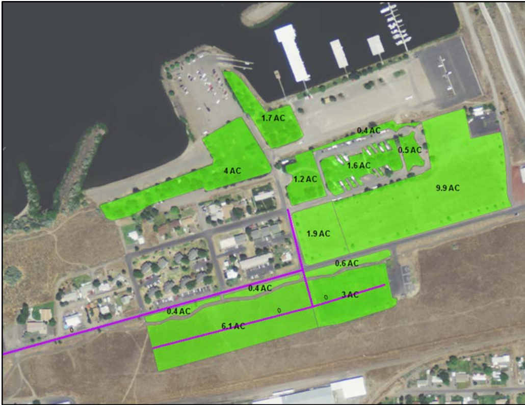
Figure 2.3 – 0.8 mgd Reuse Water Option: Marina Park Irrigation
