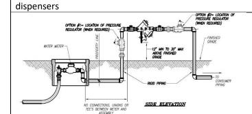
REDUCED PRESSURE BACKFLOW ASSEMBLY These are typically **above ground in an insulated box or in a mechanical/maintenance room**. Typical applications would be for car washes, breweries, industrial plants, laboratories, laundries, wells, concrete plants, medical/dental facilities
