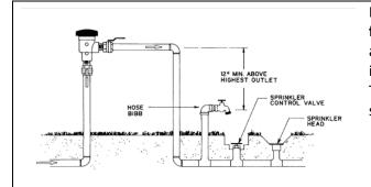
PRESSURE VACUUM BREAKER These are typically found near a house or building and will be above ground at highest point on lot. This installation shows a sprinkler system application. Typical applications would be for irrigation sprinklers.
